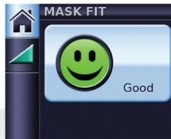
3. If necessary, adjust your mask, mask cushion and headgear until you have a Good mask-fit. After three minutes, the pressure reverts to the set pressure and treatment will begin. You can end mask-fit at any time by pressing
