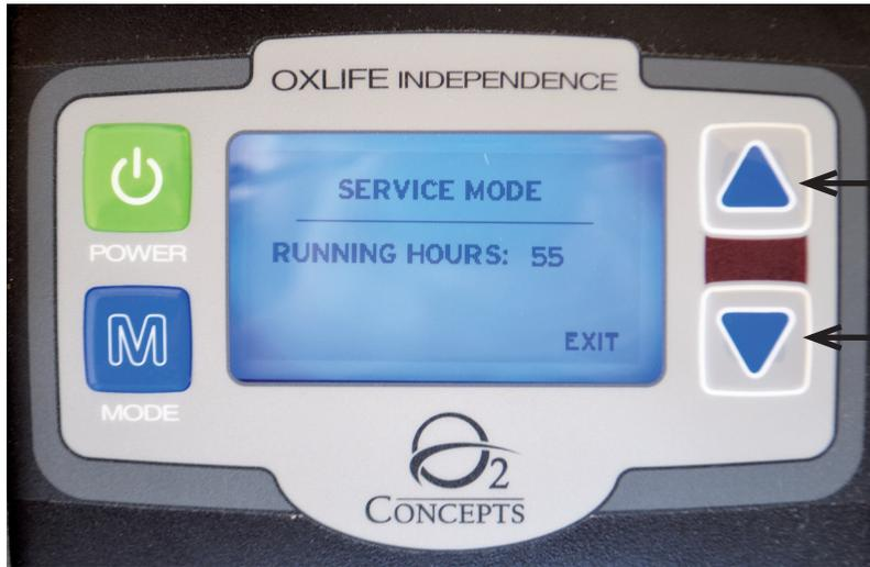
From Main Operation Screen – Press both Blue Up and Down Arrows simultaneously to access Service Mode screen.
