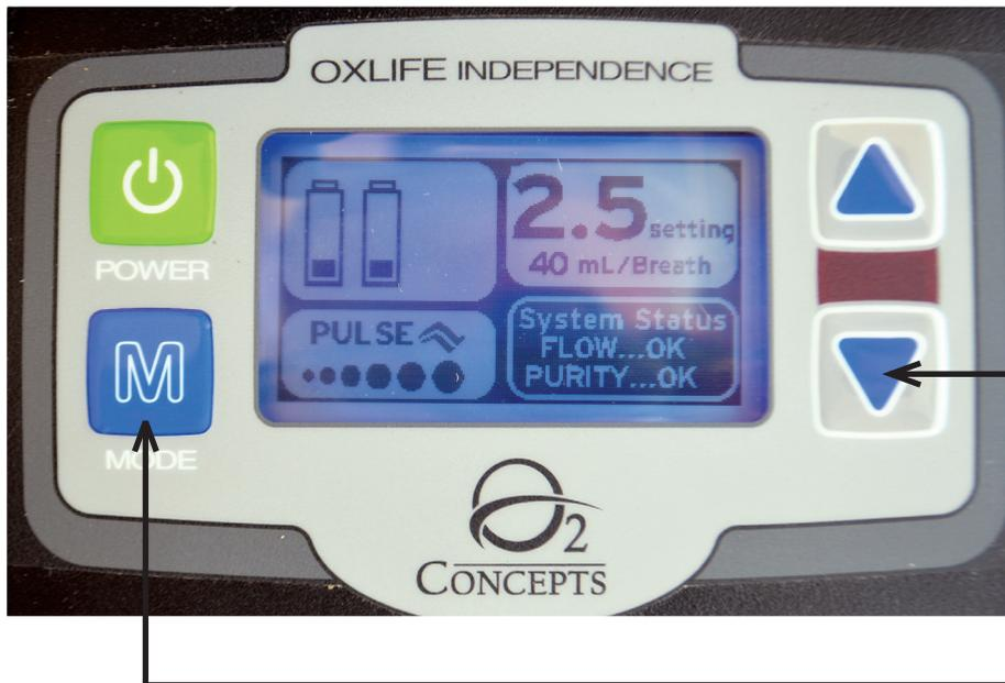
Press blue Mode button and blue Down Arrow simultaneously to access Engineering Screen
