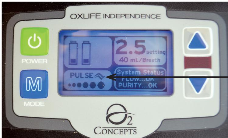
In Pulse Flow Mode – the wave symbol will appear each time a bolus of oxygen is delivered to the patient.
