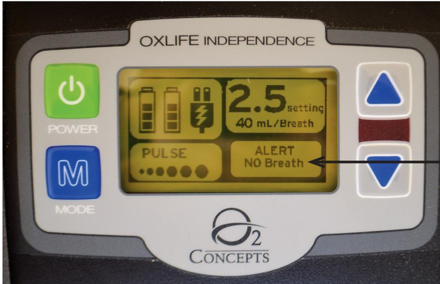
Alerts will display in the lower right corner of display screen. The screen will turn Yellow or Red depending on the type of alert.
