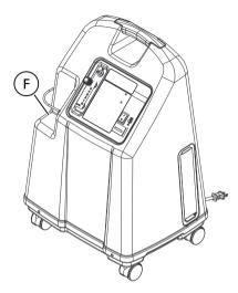
6. When placing the humidifier bottle in the compartment **(F)** on the concentrator, attach the humidifier bottle/adapter tube **(H)** to the oxygen outlet connector **(I)** on the concentrator.
