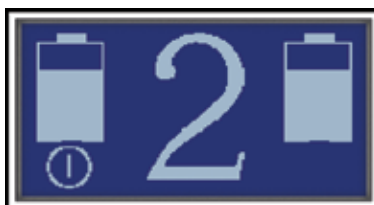
Figure 9. Touch the number to change the flow setting.
