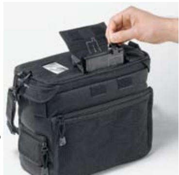
Figure 4. Inserting the secondary battery.
