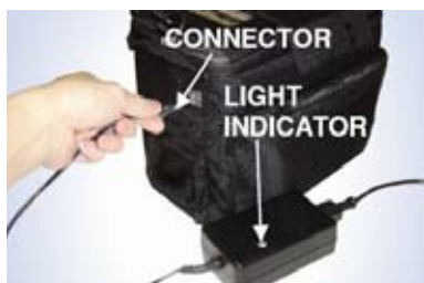
Figure 6. Connecting the power cord to the connector located under the Velcro flap. A typical battery charging screen is shown on the right
