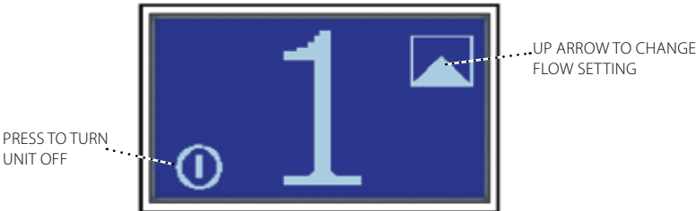
Figure 16. To change the flow setting, touch the setting number. (Here, it is the number 1.) This causes the up flow change arrow to appear. To increase the flow setting, press the up arrow until you reach your prescribed setting. The flow setting arrow disappears 5 seconds after you touch it. For another example of the flow change arrows, see the next figure.
